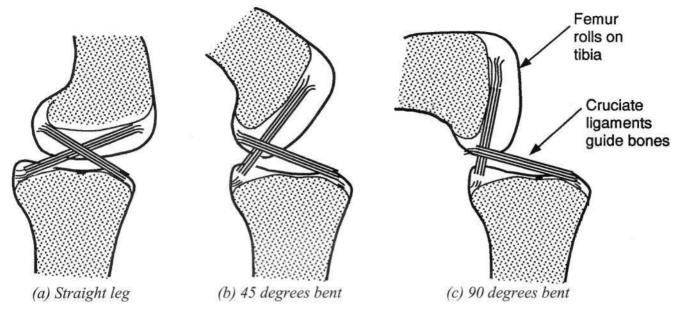
Figure 2, The irreducible mechanism of the knee (bones cut away to show cruciate ligaments).
