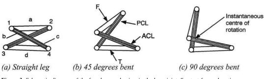
Figure 3, Schematic diagram of the four-bar mechanism in the knee joint. See text for explanation.
