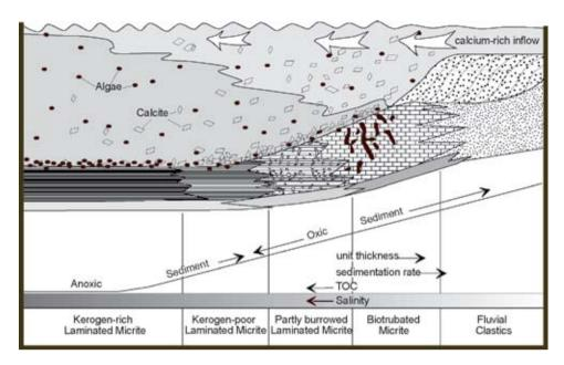
**Figure 33.** A depositional model for Fossil Basin developed by Buchheim and Eugster.<sup>27</sup> The model explains the lithology and distribution of laminated sediments in Fossil Lake.
